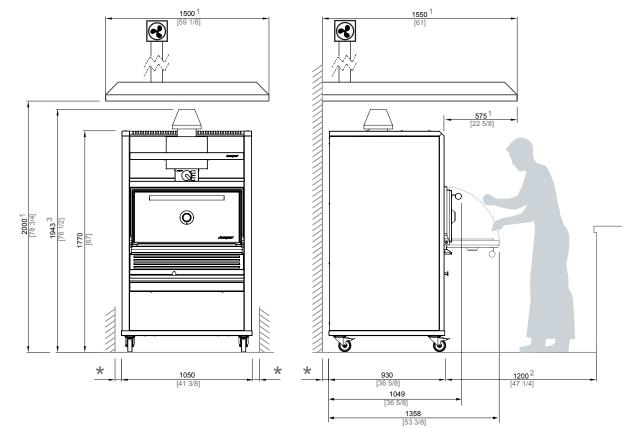
\* MINIMUM DISTANCE TO FLAMMABLE ELEMENTS: 300 mm [12 in] / RECOMMENDED DISTANCE TO ANOTHER ELEMENTS: 100 mm [4 in]
