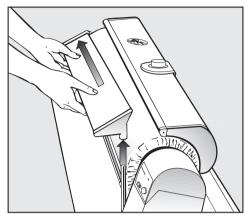
■ First remove the feed-in table by lifting it out of the right hand holder, and then pulling it out to the left of the roller.
