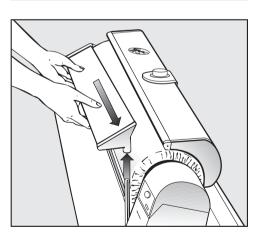
■ Remove the feed-in table as described in the section "Ironing".
